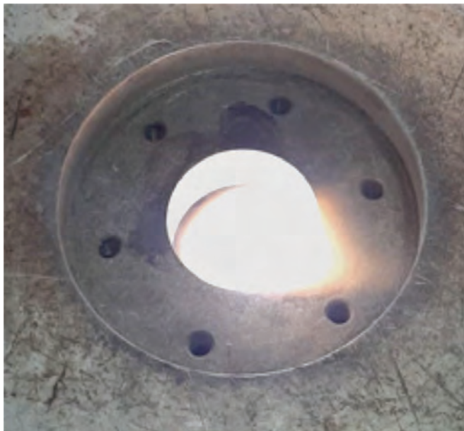
Figure 7. Thermal runaway phenomenon followed by microwave plasma.
