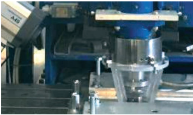
Figure 12. Enclosure for shielding gas supply (FSW-IG).
