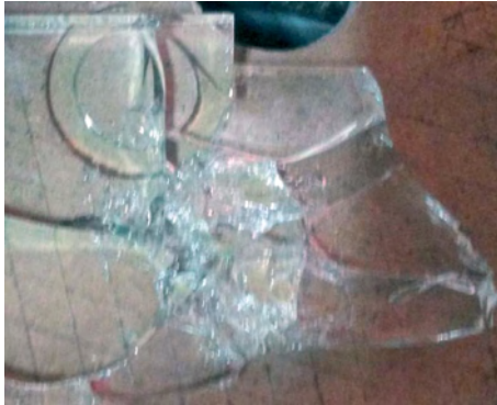
Figure 8. Cracks of the glasses.
