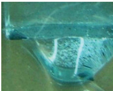
Figure 9. Glasses joined using hybrid MW-R procedure.
