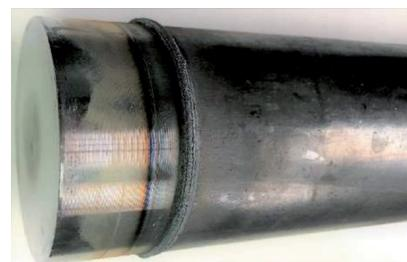
Figure 4. Welded joint pipe with bottom.
