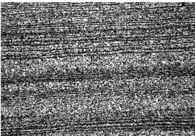
Figure 16. Microstructure (x200) of base metal of the pipe
