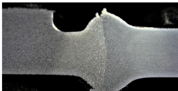
Figure 11. Macro section of the welded joint.
