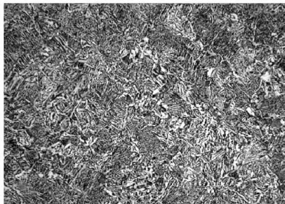
Figure 13. Microstructure (x200) of the overheating area on the bottom side.
