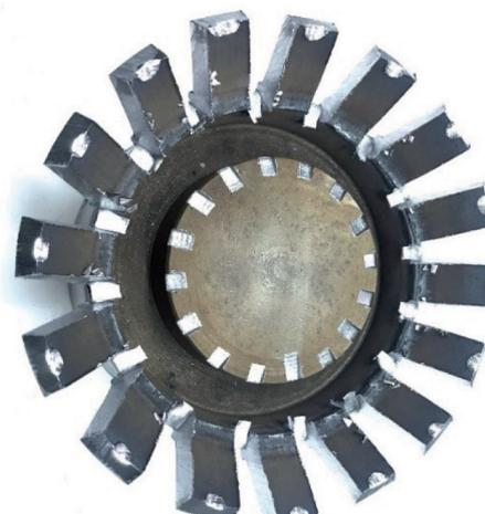
Figure 6. Results of bending tests of welded joint.
