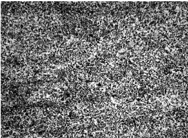
Figure 15. Microstructure (x200) of the area of complete and incomplete recrystallization on the pipe side
