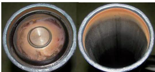
Figure 3. Surfaces of butts pipe and bottom are covered with a layer of melt metal before upset.
