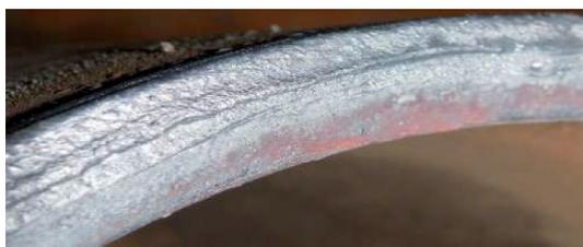
Figure 2. Traces left by welding arc during heating of the outer edge pipes.
