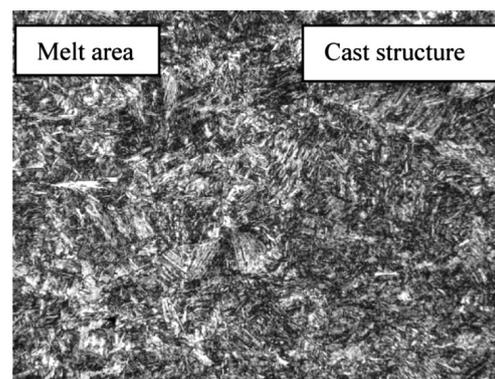
Figure 8. Microstructure (x200) of cast metal and melt area.
