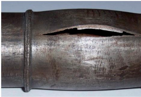
Figure 7. Hydraulic pressure tests result of weld joint.
