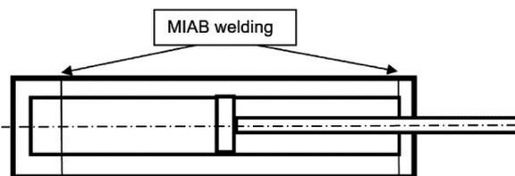
Figure 5. Application MIAB for welding hydraulic cylinder.
