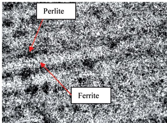
Figure 9. Microstructure (x200) of the area of complete and incomplete recrystallization on the bottom side.
