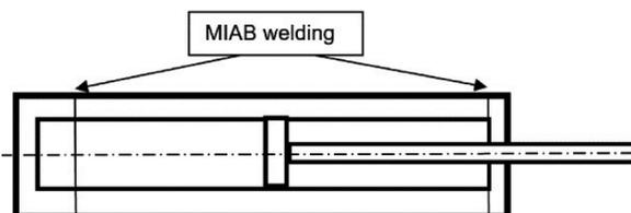
Figure 5. Application MIAB for welding hydraulic cylinder.
