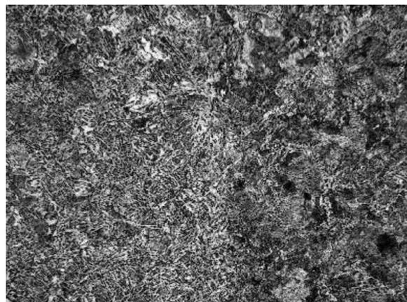
Figure 12. Microstructure (x200) of welded joint.
