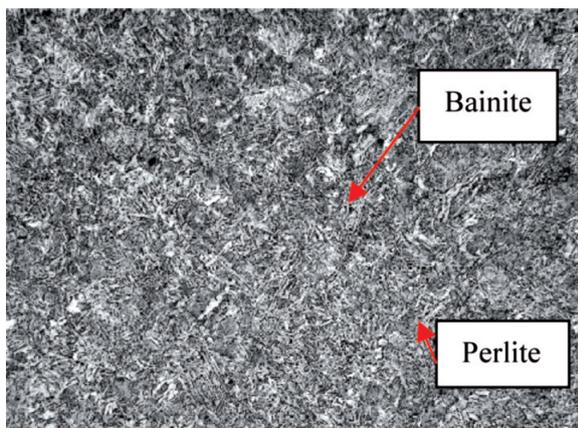
Figure 10. Microstructure (x200) of the overheating area on the bottom side.
