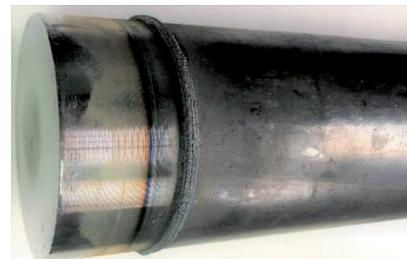
Figure 4. Welded joint pipe with bottom.
