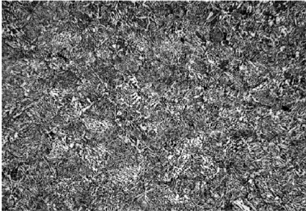
Figure 14. Microstructure (x200) of the overheating area on the pipe side.
