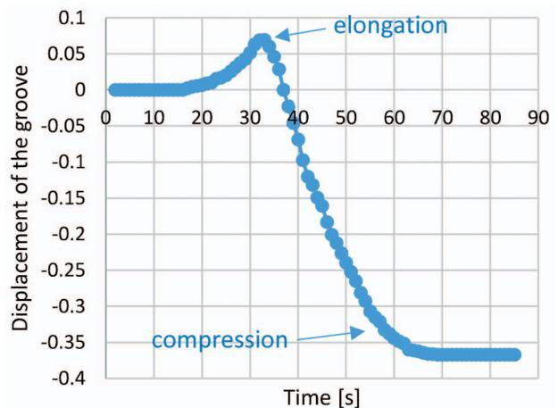
Figure 7. Deformation by welding sequence.
