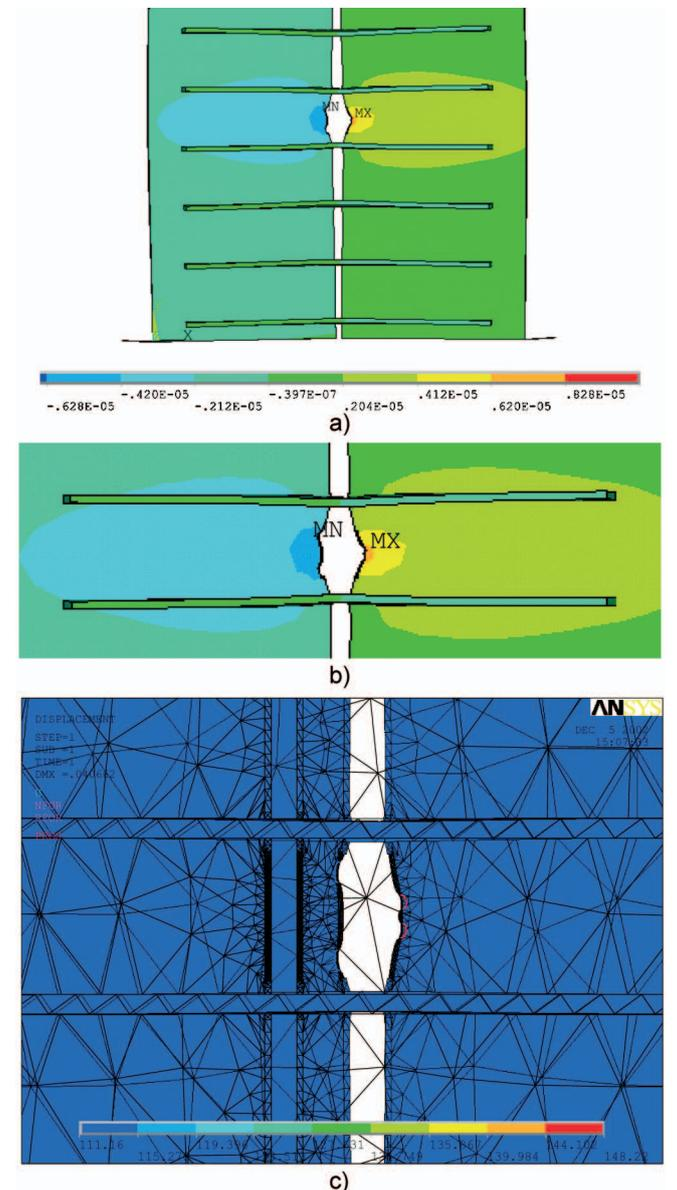
Fig. 4 Geometrical model connected with compression bars (a.) and the displacement error given by the compression bars (b.)
