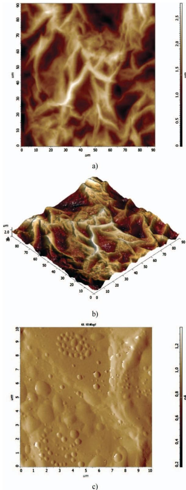
Figure 4. AFM images (AC mode) of the paraffin film surface. a) 2D AFM image of the surface morphology (90  $\mu\text{m}$  scan size); b) 3D rendering of the area imaged in a); c) amplitude (error) signal revealing fine details in a) (10  $\mu\text{m}$  scan size).
