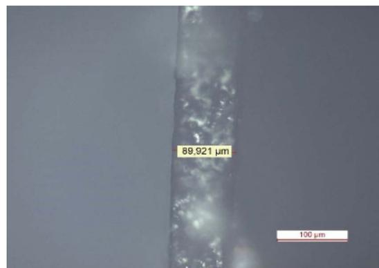
Figure 3. Optical microscopy image of the paraffin film thickness.
