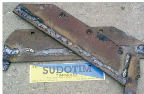
Figure 5. Plow equipped with self-sharpening modulated elements.
