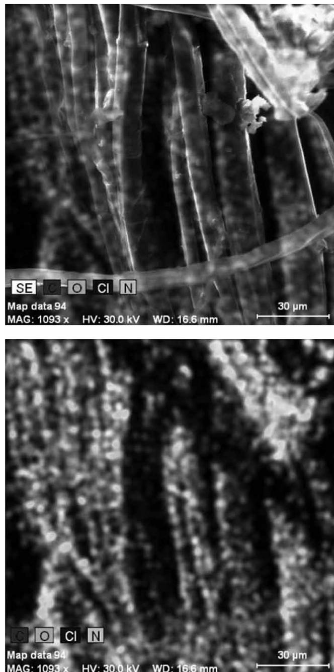
Figure 1. SEM/EDX images at X 1090 magnification for: F- reference flax support; F-MCT-β-CD grafted (functionalized) flax support.
