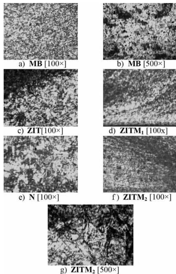
Figure 6. Microstructures in FSW joint for S 420MC.
