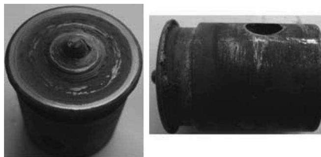
Figure 2. Deformed shoulder of the welding tool, after 20-30 mm of weld.
