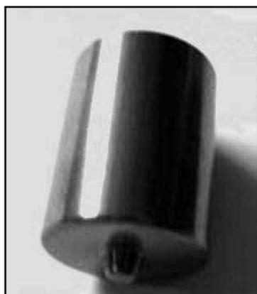
Figure 1. Welding tool with smooth tapered pin and smooth shoulder.
