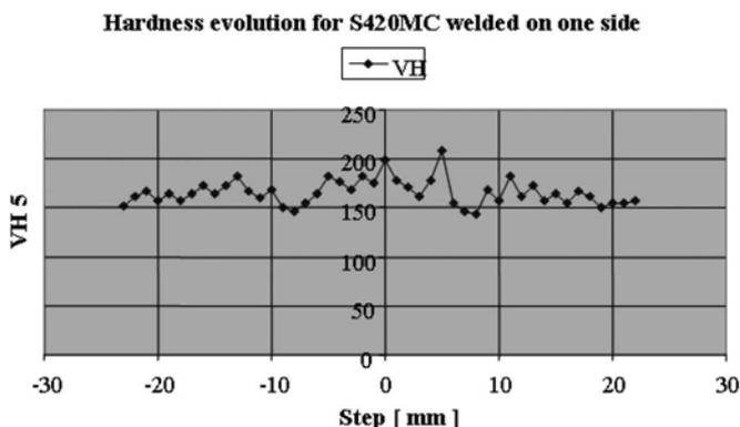
Figure 7. Hardness evolution for S420MC welded on one side.
