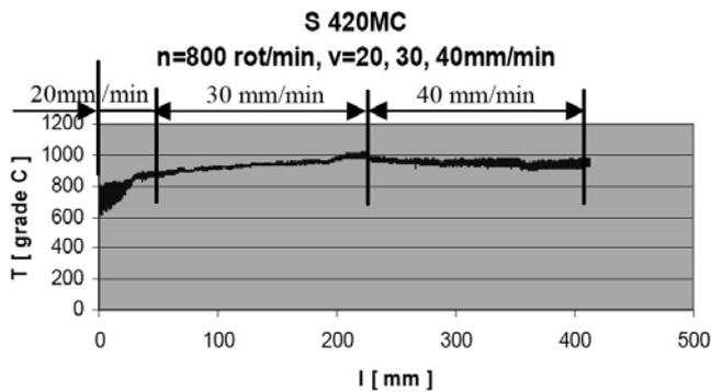
Figure 4. Temperature evolution recorded with thermographic camera.
