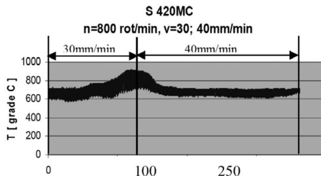
Figure 9. Evolution of temperature monitored by thermographic camera.
