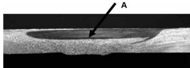
Figure 5. Macroscopic analysis of S420MC - friction stir welded on one side.
