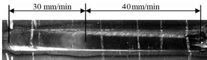
Figure 8. Joint aspect for S 420MC welded on both sides.
