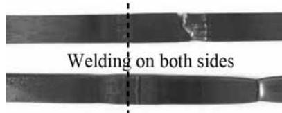
Figure 13. Aspects of FSW welded samples, on both sides, after static tensile test.
