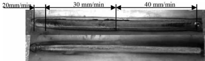
Figure 3. The aspect of welded joint on one side for S 420MC.
