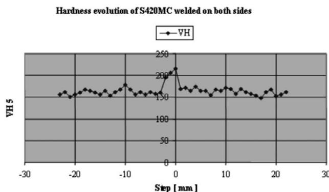
Figure 11. Hardness evolution for friction stir welded joint on both sides of steel S 420MC.
