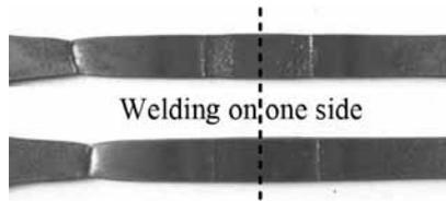
Figure 12. Aspects of FSW welded samples, on one side, after static tensile test.
