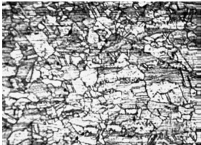
Figure 7. Microstructure of the heat affected zone (MO, 100x).
