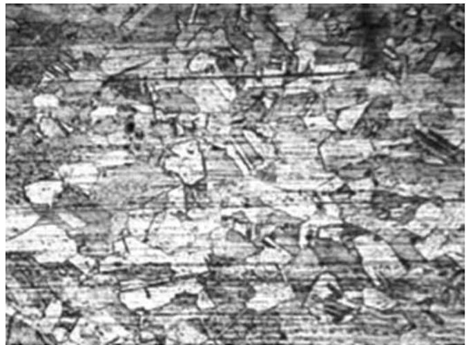
Figure 6. Microstructure of the base metal (MO, 100x).
