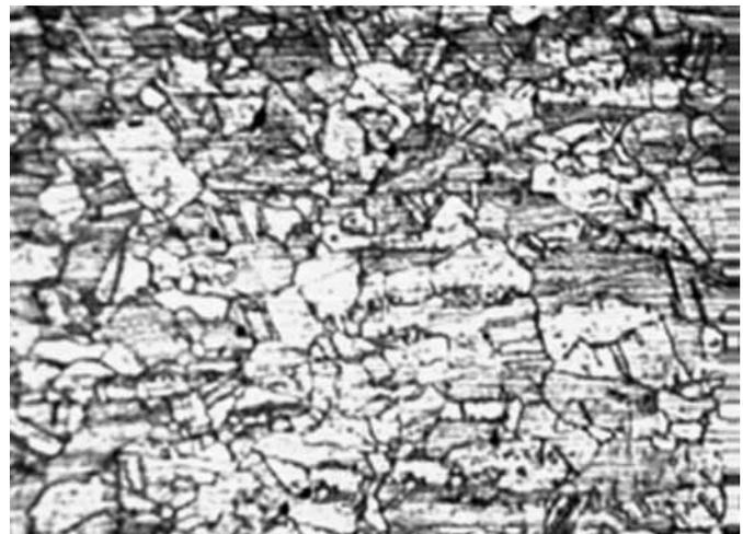
Figure 7. Microstructure of the heat affected zone (MO, 100x).
