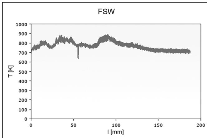
Figure 4. Variation of the temperature during the FSW welding process of Cu99.
