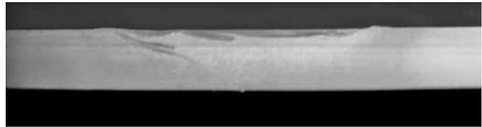
Figure 5. Macrostructure of the FSW welded joint of Cu99.
