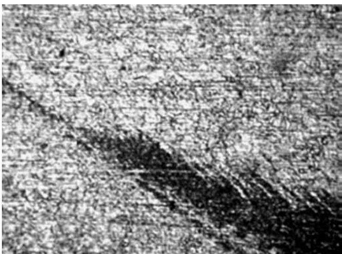
Figure 9. Microstructure of the zone affected by both heat and strain (MO, 100x) on the advancing part of the tool.
