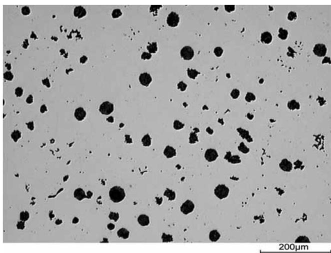
Figure 4. Nodular graphite form of the flange material.
