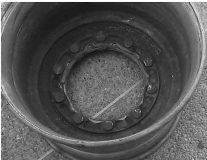
Figure 1. View of the wheel with broken off flange crown.
