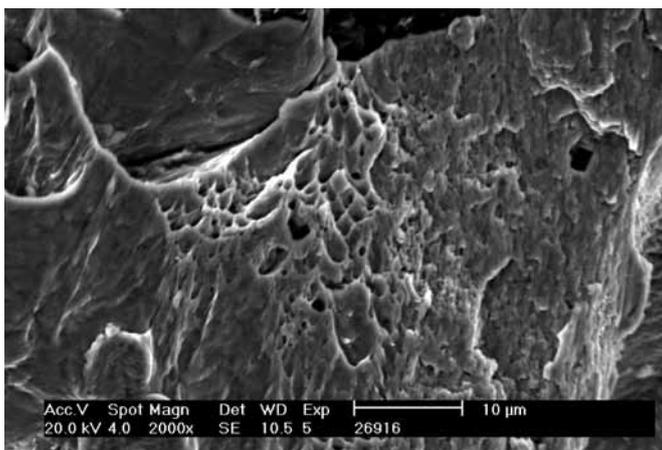
Figure 8. Final fracture zone at high magnification.
