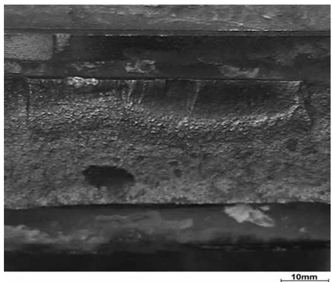
Figure 3. Close-up of the fracture surface of the flange.
