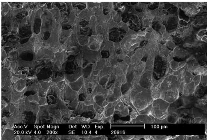
Figure 7. Final fracture zone at low magnification.
