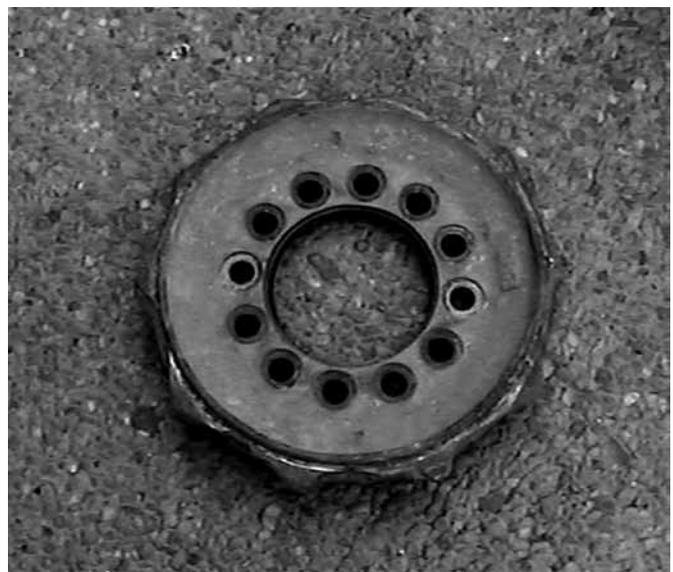
Figure 2. View of the failed flange – the crown is broken off.
