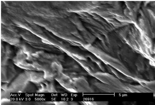
Figure 6. Fatigue striations found in the fatigue zone of the flange fracture surface.
