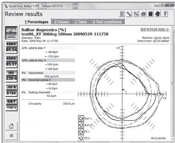
Figure 4. QC10 ball diagram without the NC axis
