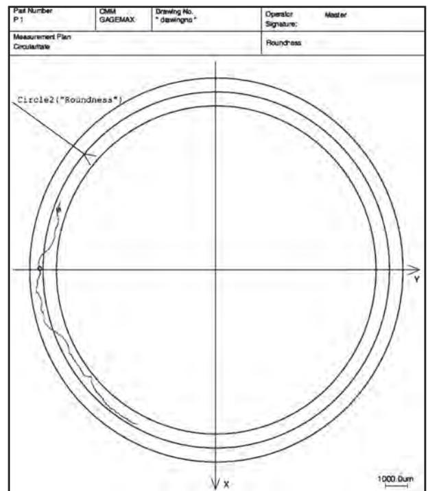
Figure 10. Error measurement of a nibbled part
