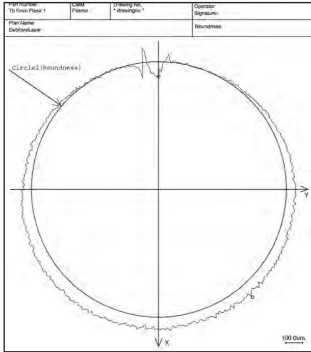
Figure 8. Errors for speed of 1500 mm/min and  $K_{PD}=19.69$
