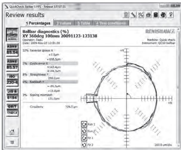
Figure 5. QC10 ball diagram with the NC axis tuned controller
