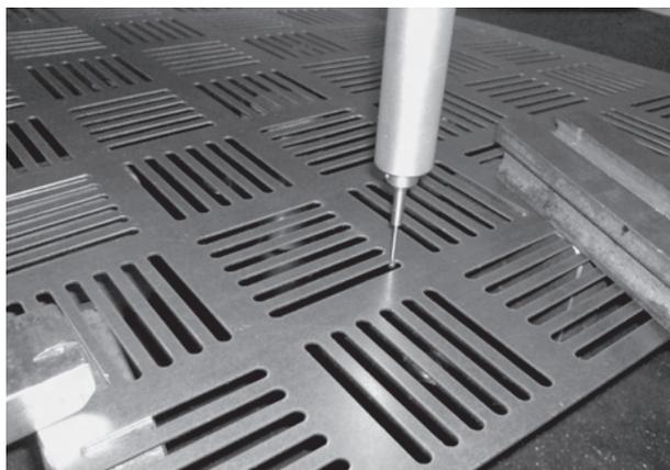
Figure 1. Snapshot during measurement on Prismo 7 S-ACC
