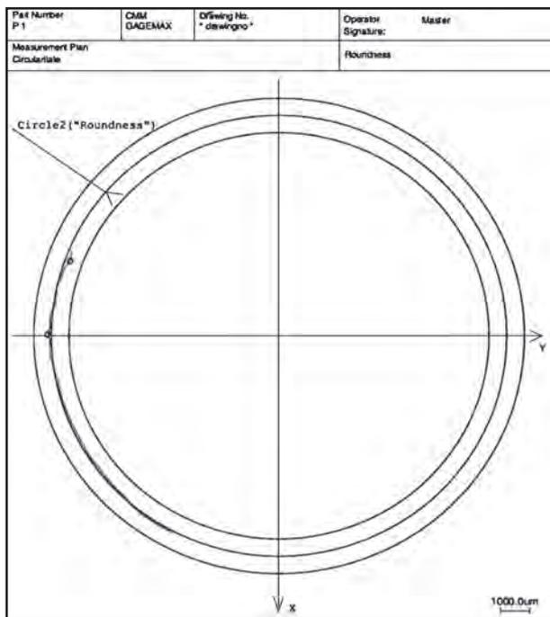
Figure 11. Error measurement of a nibbled part with tuned system parameters
