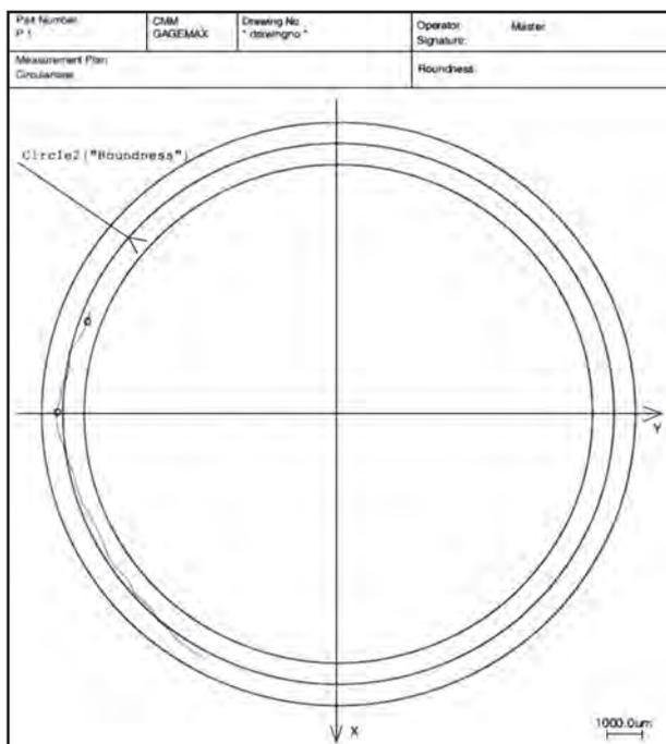
Figure 12. Error measurement of a nibbled part with tuned system parameters and speed of 30 m/min
