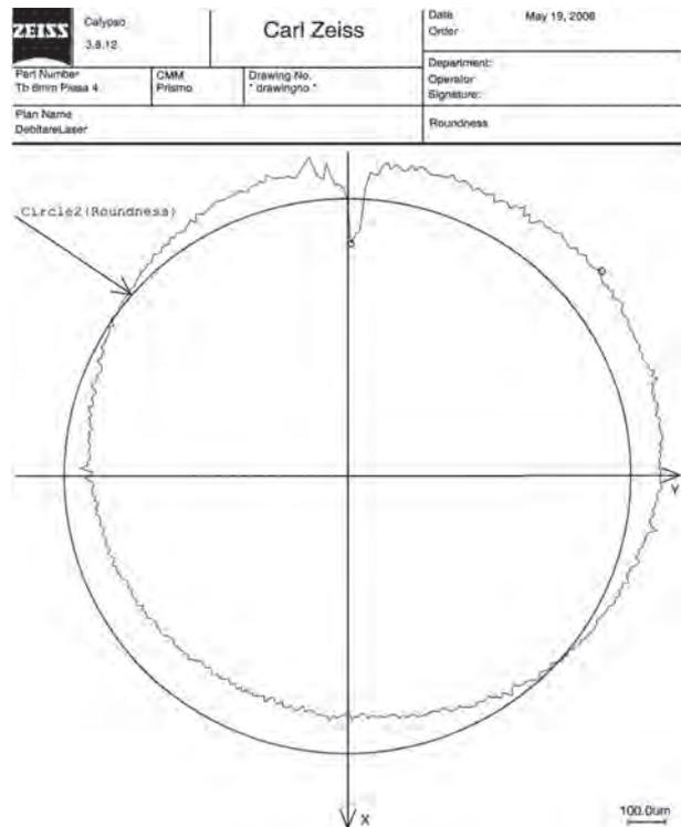
Figure 6. Errors for speed of 1500 mm/min and  $K_{PD}=38.38$
