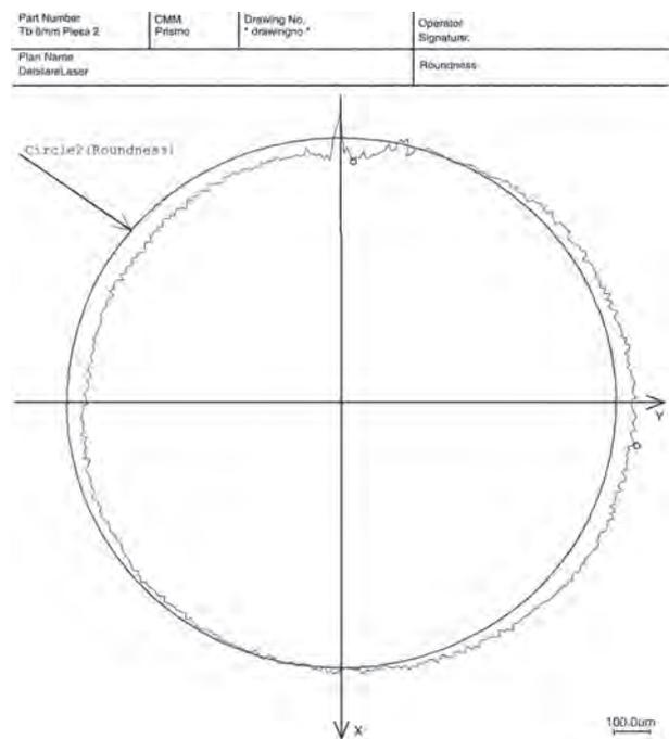
Figure 7. Errors for speed of 800 mm/min and  $K_{PD}=19.69$
