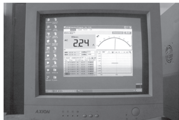
Figure 5. Indicator dial of the virtual measuring instrument results, monitor of the computer (10). In the Figure 4 the electronic multimeter type UT70B is shown, with RS 232 interface for data acquisition on the computer, where the measured extents
