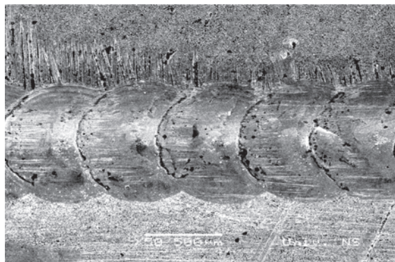
Figure 1. Laser welded joint – laser process parameters: pulse energy 48J, pulse duration 6.0ms, frequency 5.5 Hz [10]
