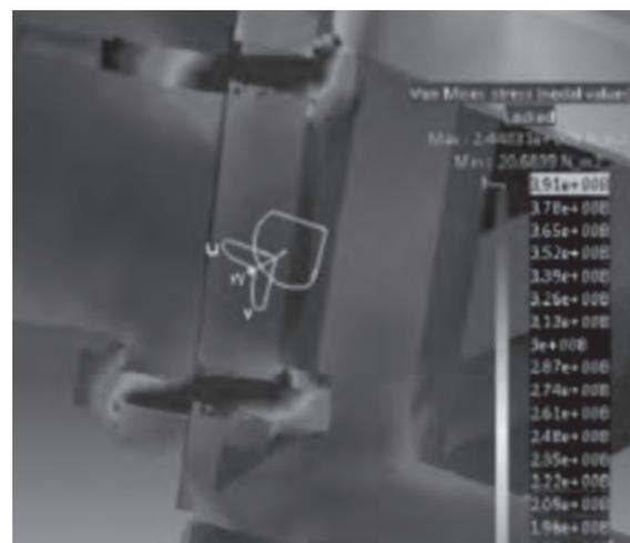
Figure 12. Chassis screws connection with the bus turntable in the unmodified state with a given value of stress. wedges. Combined loads are visible and uneven distribution of stresses in the stem screw. The dominant loads are shearing and pulling, stretching, bolts. In Figure 13 is shown, the analysis
