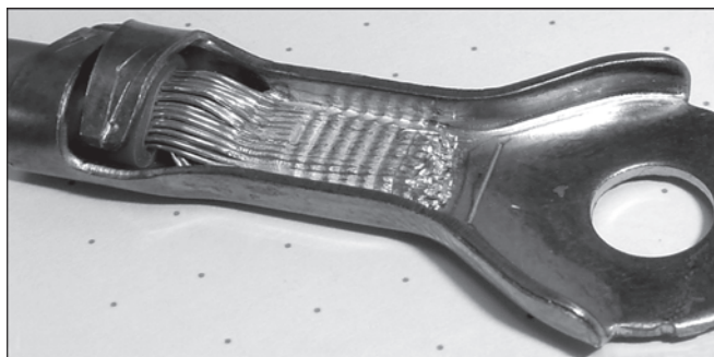
Figure 11. Eterogen joint Al+Cu of the type plate-strand, welded US
