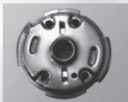
Ultrasounds welding, 4 rivet joints, PC + 6 % fiber in automotive micromotors
