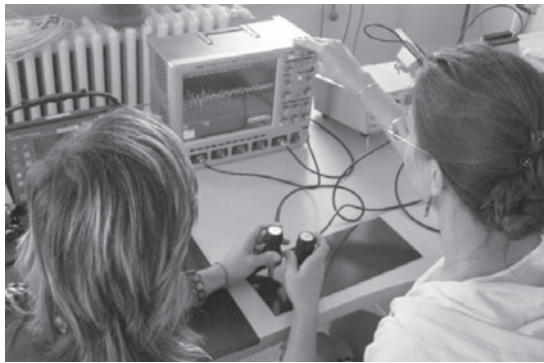
Figure 4. Ultrasound with Hertzian contact experimental set-up.
